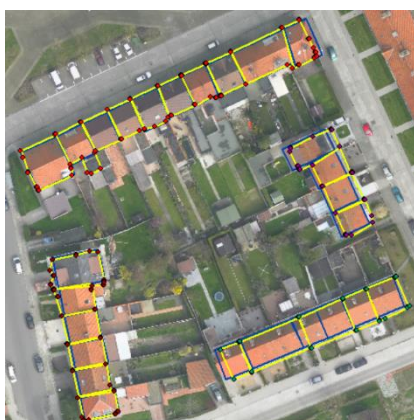
Figure 12 . Digitized footprints in ArcGIS (blue) and extracted footprints by algorithm (yellow)
