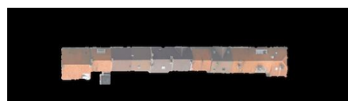
Figure 7 . Rotation of building block to the inverted complement of angle of the dominant direction
