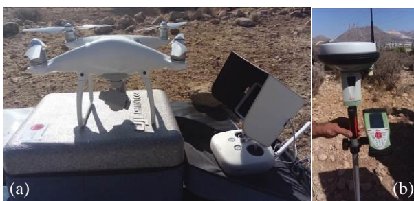
Figure 4. The DJI Phantom-4 unmanned aerial vehicle was used for image acquisition in this study (a), Leica GS10 global position system with dual frequency was applied to collect ground control points (b) (Photo taken by A. Chenrai).
