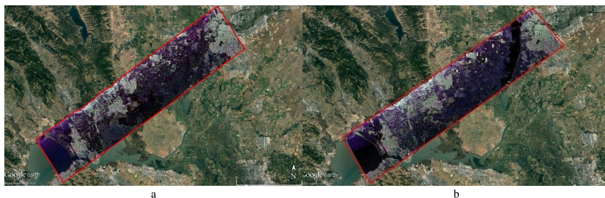
Figure 1 Georeferenced and multi-looked Pauli images in Google Earth software. a) 2014 data – b) 2017 data
