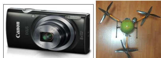
Figure 3. Air platform (hexacopter) and preferred sensor (Canon IXSUS 160)
