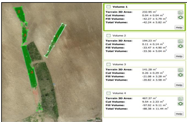
Figure 3. Calculation of cut volume of ephemeral gully by Pix4D.
