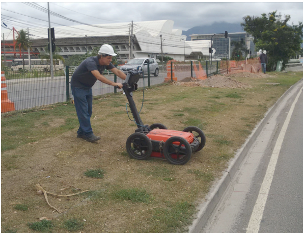
Figure 2. Ground-penetrating radar survey in progress (image courtesy of Geovoxel).
