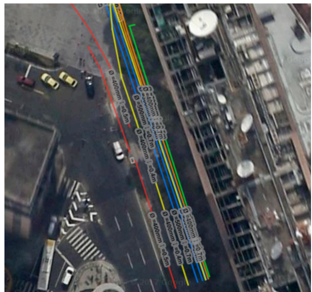
Figure 11. An example of an agglomeration of buried infrastructures in the same avenue discovered by the GPR survey.
