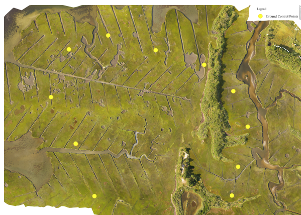
Figure 4. Differentially Corrected Ground Control Points
