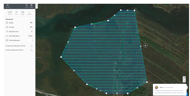
Figure 3. Low Tide Drone Deploy Flight Plan
