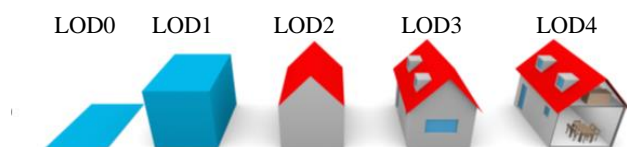
Figure. 2. A building model in CityGML LOD0 – LOD4 (Biljecki et al., 2014a).
