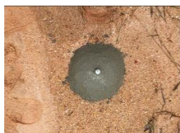
Figure 13. The example of control points established
