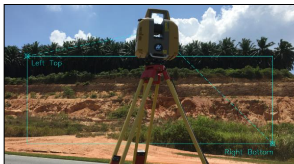
Figure 25. Determine scanning area
