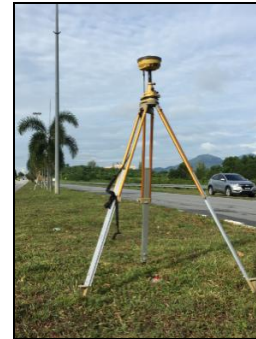
Figure 10. Topcon Hiper V GNSS receiver is used to obtain the coordinate value of observation stations
