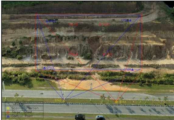
Figure 20. Scanner view of the slope taken from different scanner location which comprises of station 1 and 2
