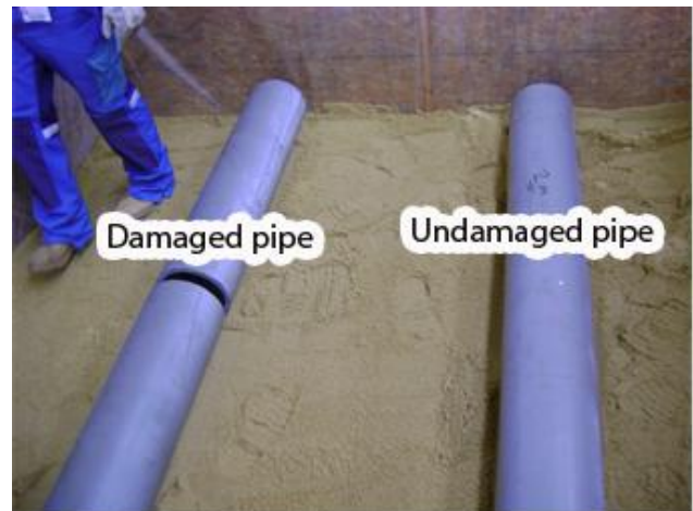
Figure 2: Arrangement of the two plastic pipes in the test box prior to burial
