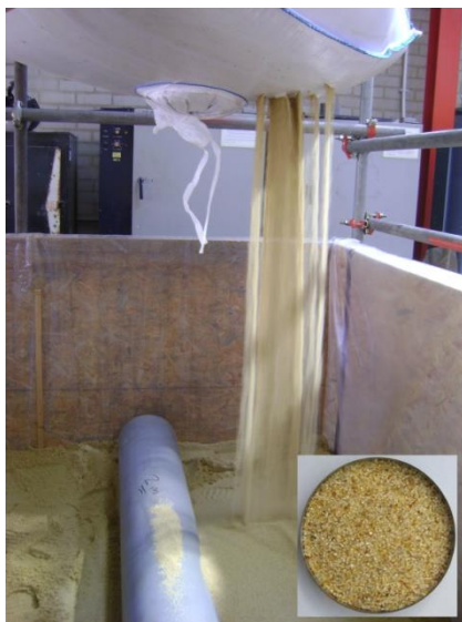
Figure 5: Fill material for test facility
