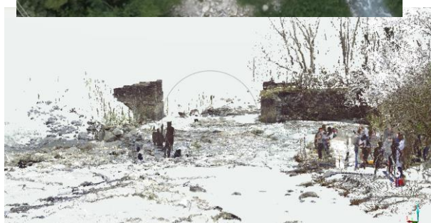
Figure 5. The ancient collapsed bridge, (above) an excerpt from the orthophoto and (below) a view of five scans registered cloud
