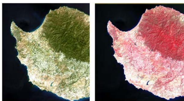
Figure 4. The city of Paphos in the year 2016: (left) Red – Green – Blue (RGB) true colour composite i.e. the band combination that corresponds to the human vision; and (right) in NIR – green – blue pseudo colour composite that enhances the presence of vegetation (in red colour).
