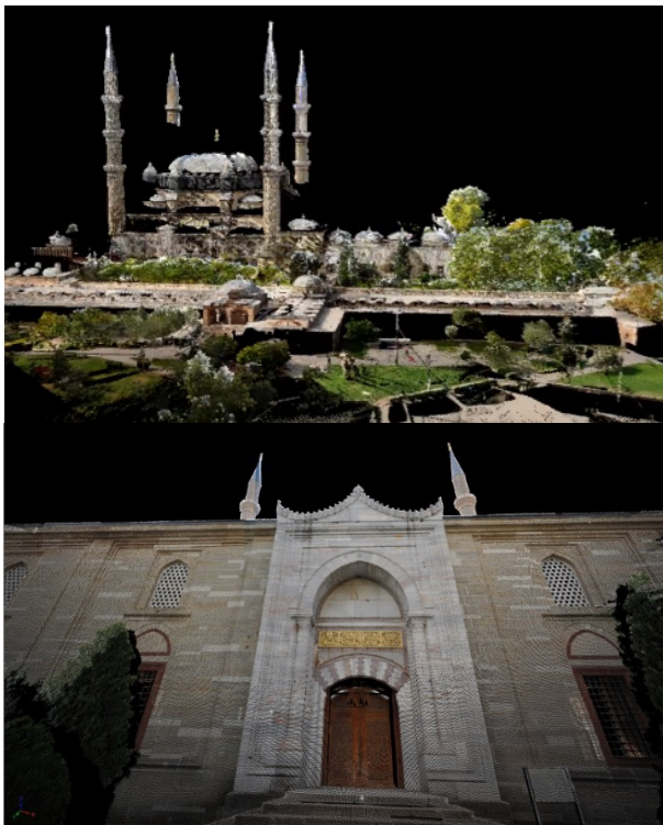
Figure 3. Part of the coloured point cloud of the Edirne mosque – overview (top) and detail (bottom)
