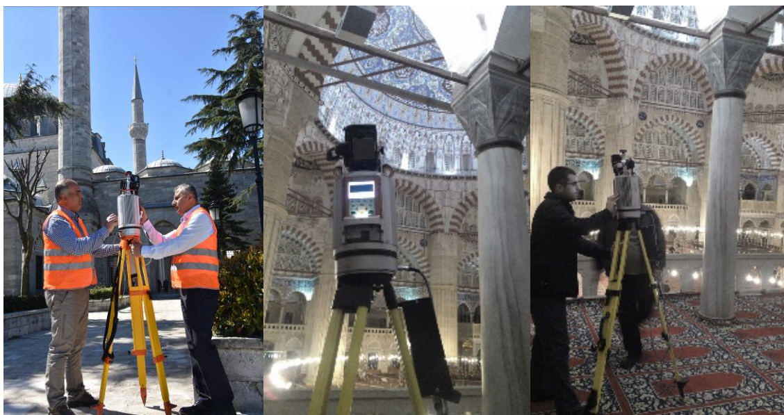
Figure 2. Data acquisition with the terrestrial laser scanning system Riegl VZ-400 on top of a minaret (left) and inside the mosque (centre and right)
