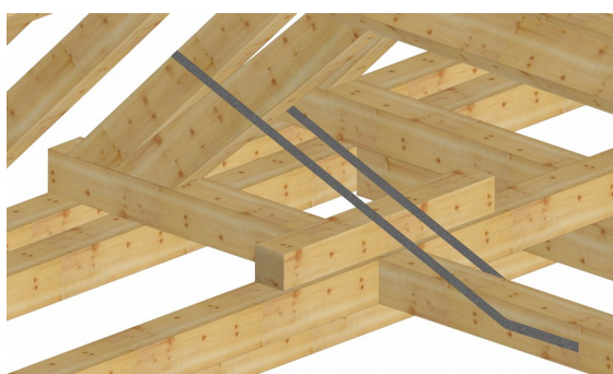
Figure 10. Photo of detail of the foot point of the Laves' balken .
