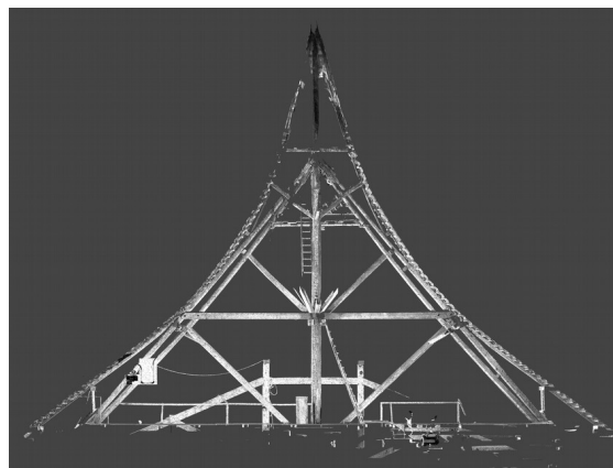
Figure 5. Longitudinal section of the pagoda. The main structural elements are extrapolated thanks to the box tool.
