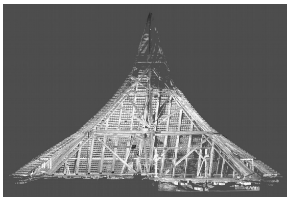
Figure 3. Section of the pagoda roof that shows the inner part of the structure.
