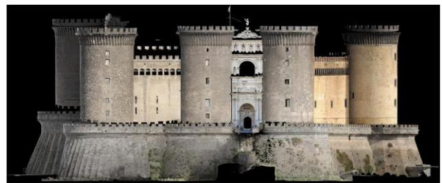
Figure 4. Real West Point Prospect Cloud Orthoprojection. Castel Nuovo.
