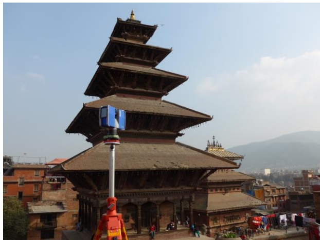
Figure 2: using a 3D scanner to record Nyatapola temple, Bhaktapur, Nepal.
