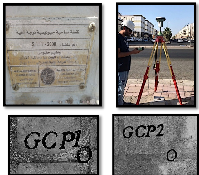
Figure 1: The process of identifying the GCPs.
