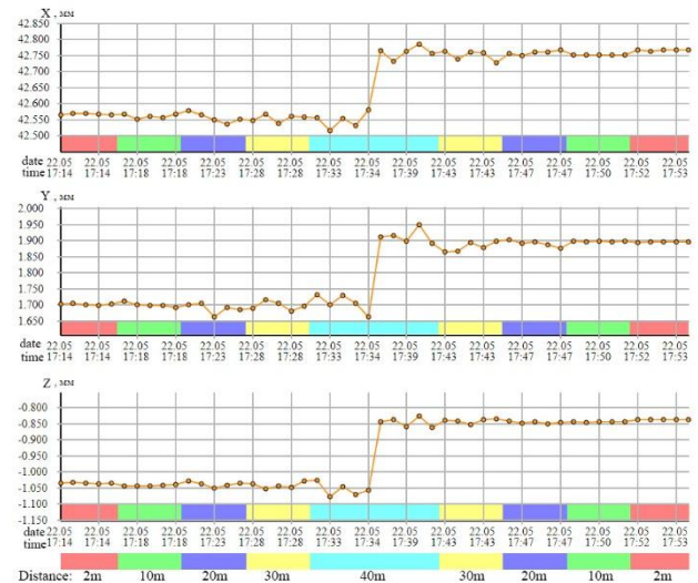
Figure 14. Relative X, Y and Z position graphs for the centers of two blocks of marks, determined by stereophotogrammetric method
