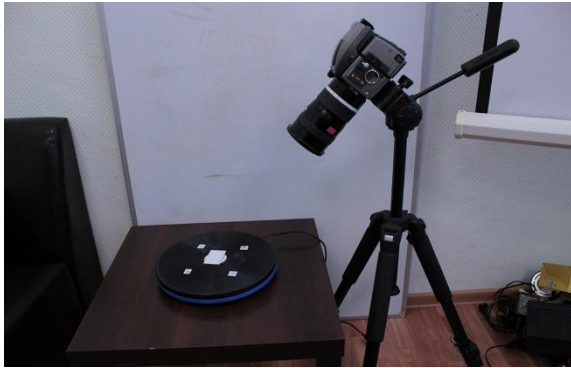
Figure 5. Calibration of the block of photogrammetric deformation marks
