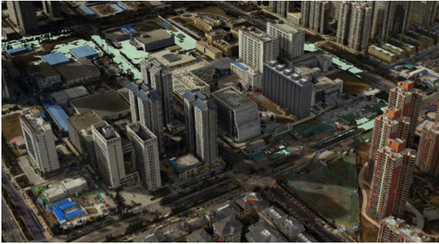
Figure 8. Rainstorm inundation scenario (simulate the scenario of heavy rain, the blue part is the flooded area)
