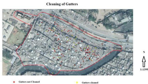
Figure 6: Cleaning of Gutters
