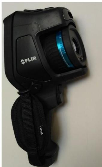
Figure 1. Thermal imaging camera Flir E95
