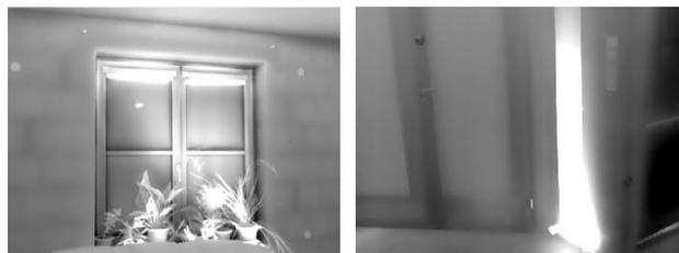
Figure 5. Left image of window is suitable for photogrammetric processing, right image of heater has lack of features and is not suitable for photogrammetric processing.
