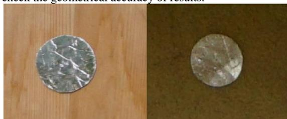
Figure 4. Aluminium targets on RGB image.
