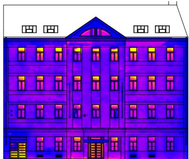
Figure 2. 2.5D model of building facade where is possible to detect certain thermal leaks.
