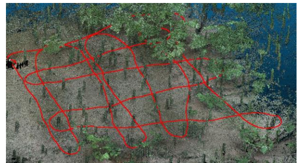
Figure 4. The specific scan path of ZEB HORIZON during the data acquisition
