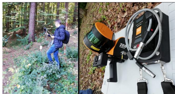
Figure 2. Left side – ZEB REVO in data acquisition process; Right side – ZEB HORIZON
