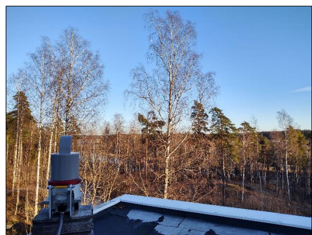
Figure 1. Test area view after data acquisition campaign in February 2020 with RIEGL VZ-2000i laser scanner facing the test area.
