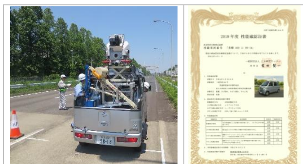
Figure 12. Developed vehicle-loading system for road surface inspection and Japanese official certification of road surface inspection
