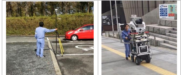
Figure 7. Typical check points (left) for evaluation of the developed trolley-loading system (right)
