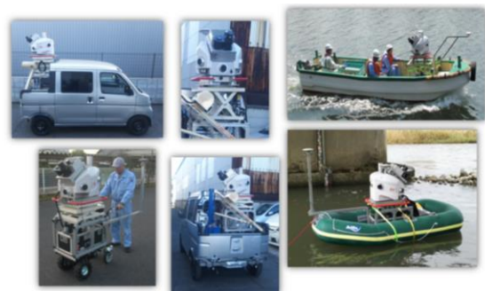
Figure 3. Developed system to achieve versatile mobile mapping
