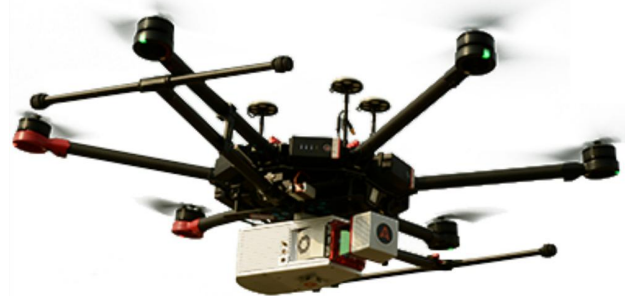
Figure 4 Dajiang M600 Pro UAV with LiDAR AS-300H.
