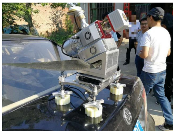
Figure 5 Vehicle point cloud data acquisition system.
