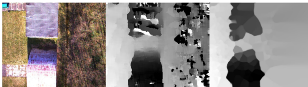
Figure 4. Densification approach: input image (left), plane sweeping (centre), interpolation (right). Image courtesy Kern (2018)
