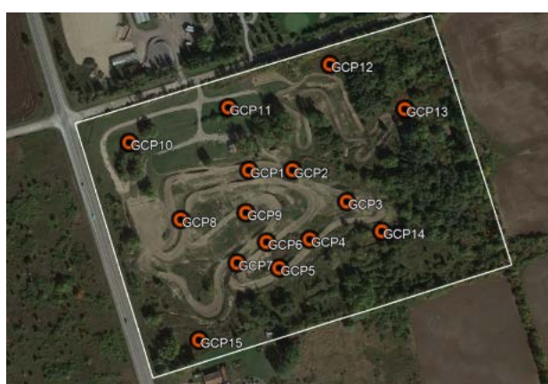
Figure 4: Applanix Test Field Showing GCP Layout
