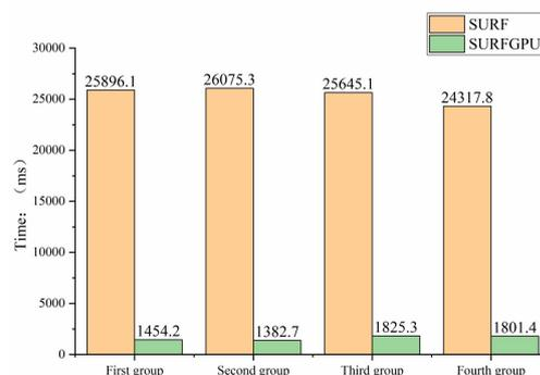
Figure 8. Comparison of operation time between SURF and SURFGPU
