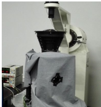
Figure 4. The geometric calibration system for PSOC measurement (left) and PSOC measurement values in 56° FOV of 910nm channel (right)
