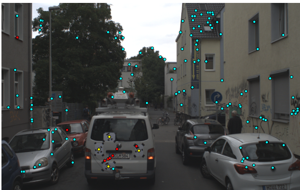
Figure 6. Image taken by the trailing vehicle at a point in time between anchor point 12 and 13; the front vehicle can be seen in the centre of the image. Yellow: observed marker points. Blue: observed tie point. Red: tie points eliminated as outliers.
