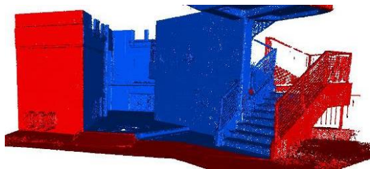
Figure 13. Point cloud showing the not considered portion (red colour) and the considered portion (blue colour) for the cloud-to-cloud distance analysis.
