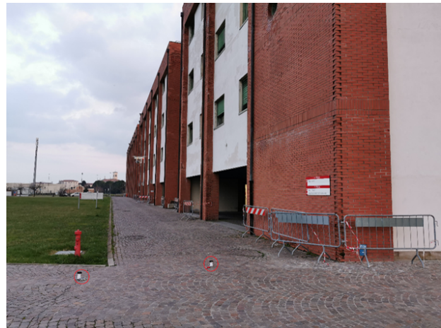
Figure 2. Pozyx UWB anchors distributed on the ground close to the building façade.
