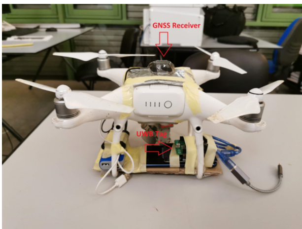
Figure 1. External sensors attached to the drone.
