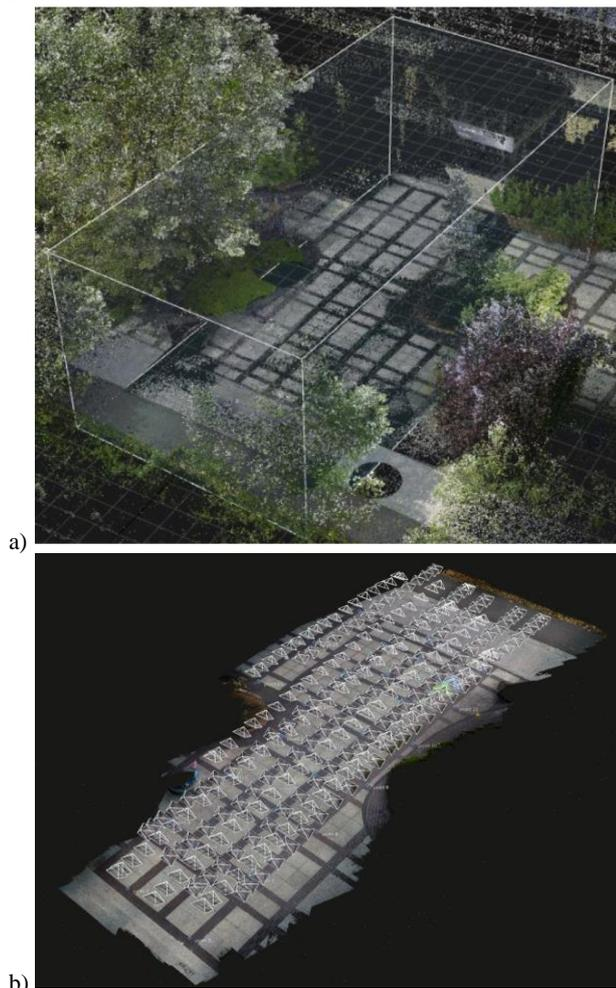
**Figure 8.** Merged TLS and dense point cloud generated from images acquired with Sony A7R III camera for test area (a), a dense point cloud generated from images acquired with Sony A7R III camera (b)
