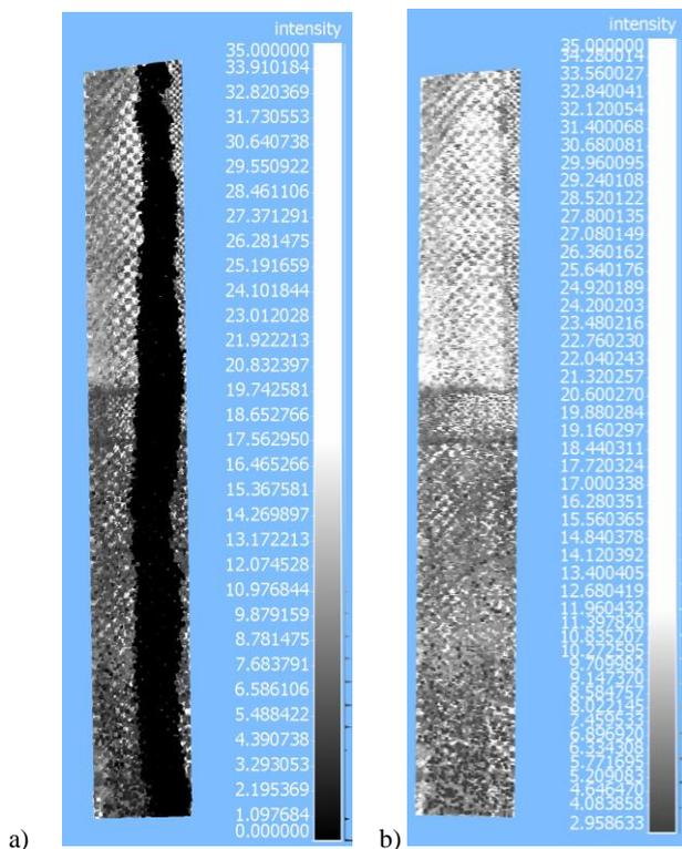
**Figure 5.** Test data acquired with Livox Avia sensor inside the building: with the noisy points (a) and with noisy points filtered out (b)
