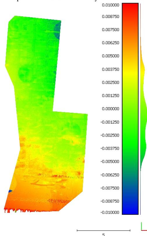
**Figure 9.** Z-coordinate differences between points clouds: point cloud only from TLS and merged TLS and image point cloud
