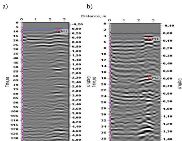
**Figure 3.** The same GPR profile obtained with two antennas: 300 MHz (a) and 700 MHz (b).
