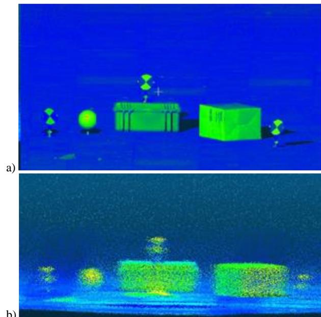
Figure 2. Comparison of point cloud quality for datasets collected with scanners: RTC360 (a) and Livox Avia (b)
