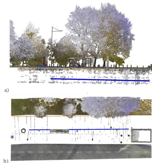
**Figure 4.** LiDAR and GPR data integration concept shows georeferenced point clouds collected with LiDAR and GPR antenna (a) indicating the water supply network showed in a top of view confirmed by manhole hatches location (b).
