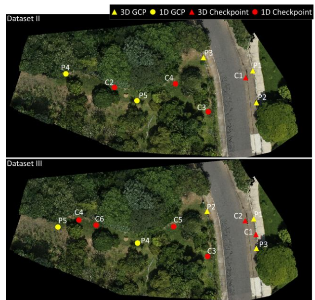
Figure 7. Top view of the generated dense point cloud that covers the test area and the localisation of GCPs (in yellow) and checkpoints (in red) used in the georeferencing process of datasets II and III.
