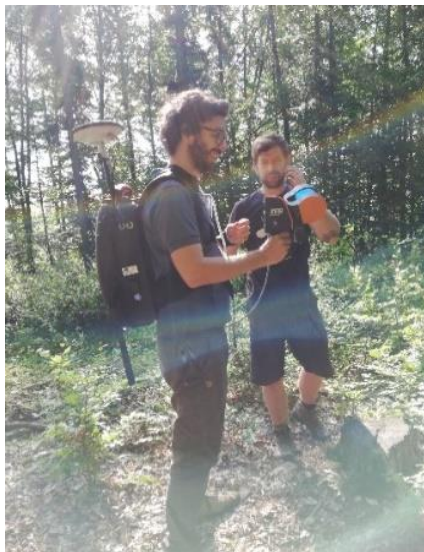
Figure 2. GeoSLAM ZEB Horizon and IMU backpack SPAN NovAtel during data collection.
