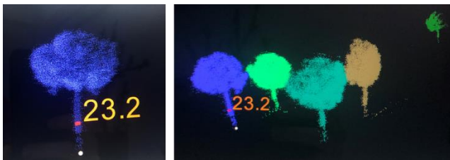
Figure 9. Example of some automatically segmented individual tree (each color represent individuality) and determining lowest position on bottom of an individual tree
