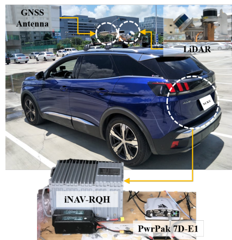
Figure 3. Experimental platform with navigation sensor configuration.
