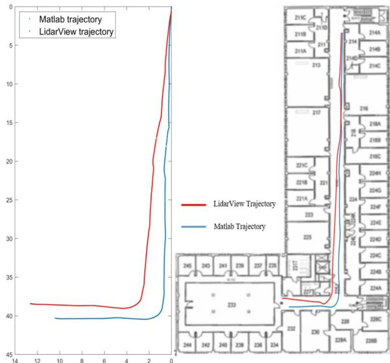
**Figure 4.** Trajectory for A-B-C corridor section, Blue line: Matlab trajectory, Red Line: LidarView (Left Side), Trajectory data matched with the underlying floor plan (Right Side)
