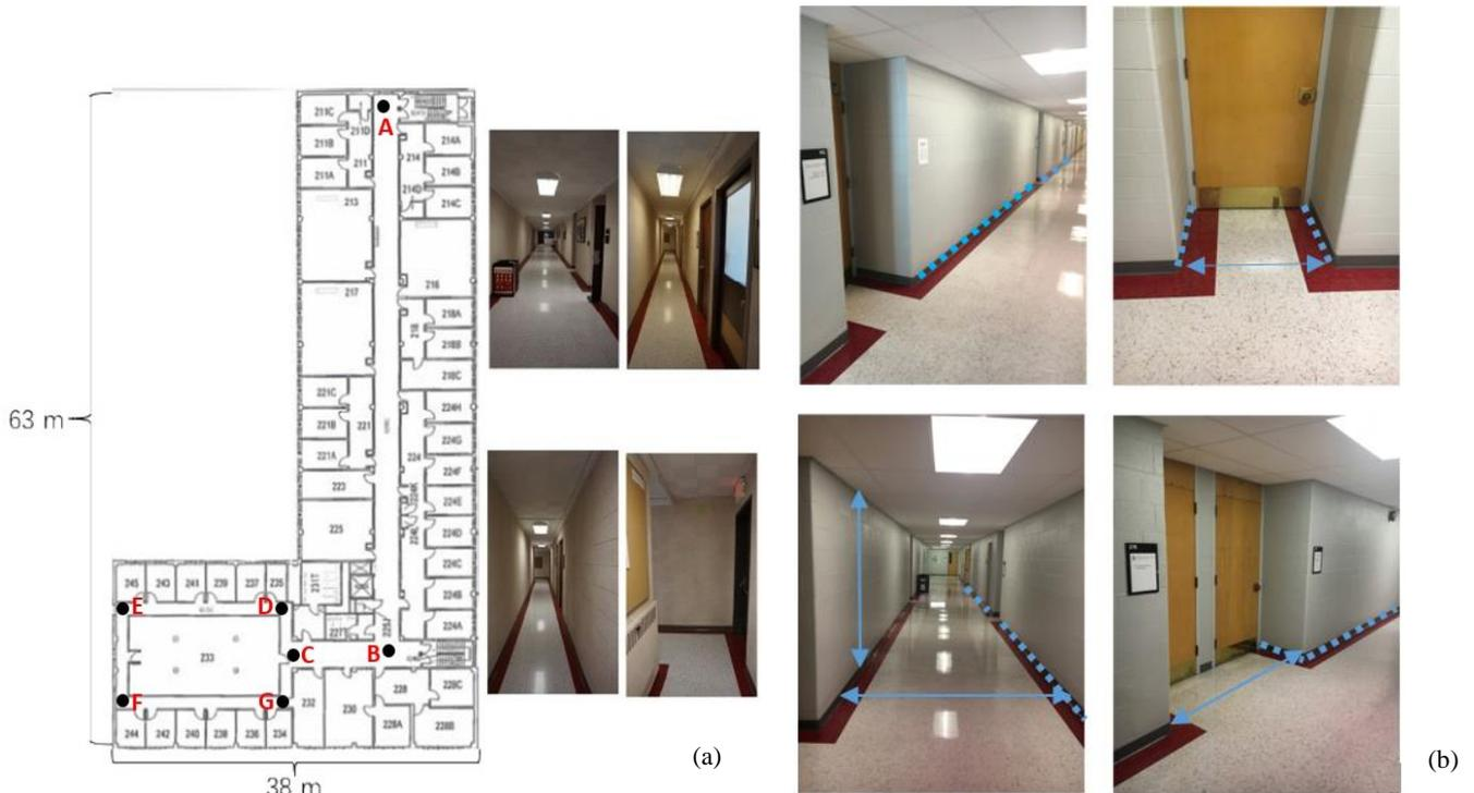
**Figure 3.** Layout for test corridor and image samples for these corridors (a) (Yuan, 2021), Key features selected for localization performance (arrows indicate corridor width and height and width of door entrances, dashed lines indicate depth of the door entrances and distances between door edges.) (b)
