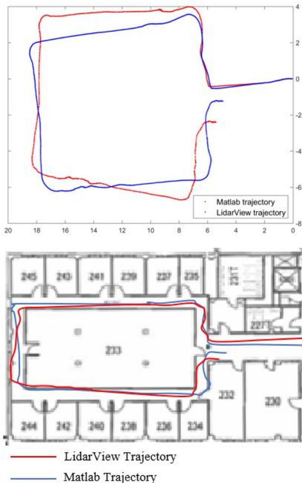
**Figure 5.** Trajectory for C-D-E-F-G corridor section, Blue line: Matlab trajectory, Red Line: LidarView (Top View), Trajectory data matched with the underlying floor plan (Bottom View)
