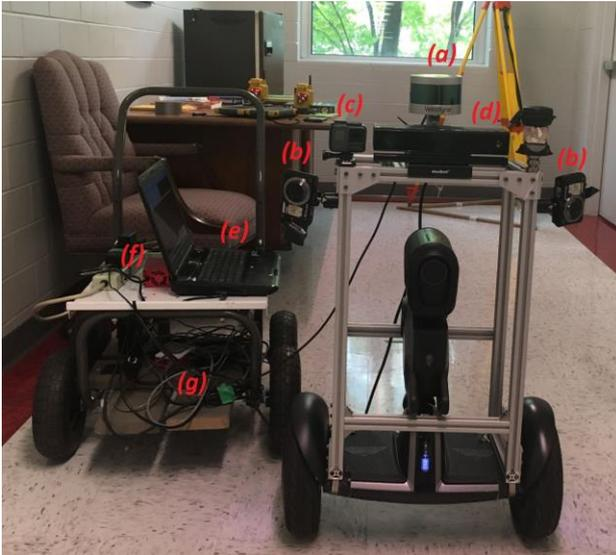
**Figure 2.** Sensors: a) Velodyne VLP-16 LiDAR, b) Casio, c) GoPro, d) Microsoft XBOX Kinect 360 Sensor; Hardware: e) Laptop, g) Raspberry pi, (f) Power Source
