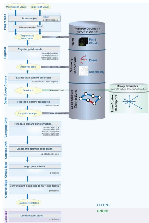
Figure 1. General workflow steps for Matlab LiDAR SLAM (Matlab 2022)
