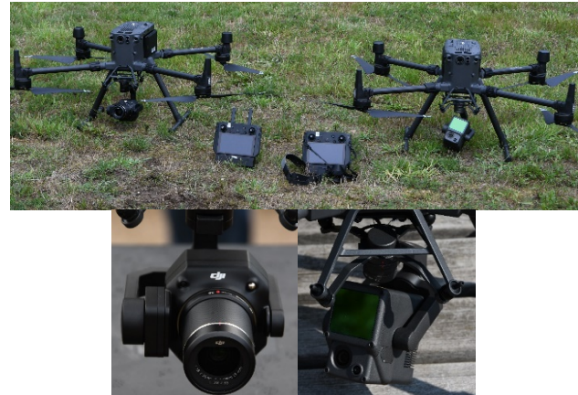
Figure 2: Top - DJI Matrice 300 RTK with Zenmuse P1 camera (left) and L1 laser scanner (right), bottom - Zenmuse P1 camera (left) and L1 laser scanner (right).
