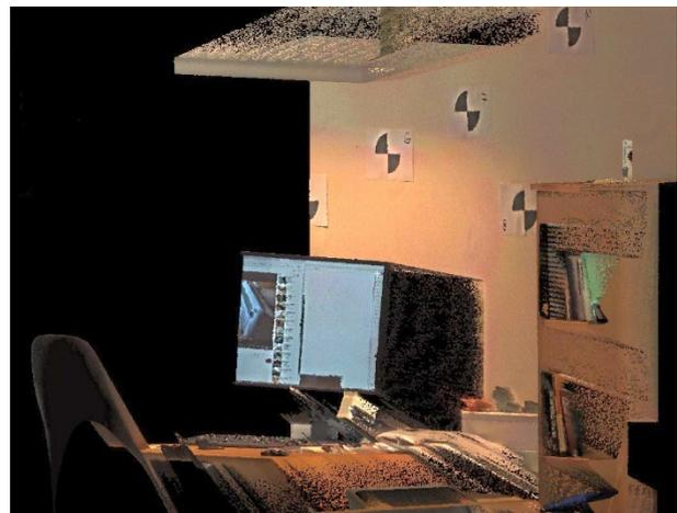
**Figure 3.** Reference LiDAR point cloud of a corner area.
