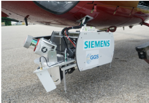
Figure 1. Sensor System for the OHL inspection used by Siemens based on 11 cameras and LiDAR mounted at a helicopter
