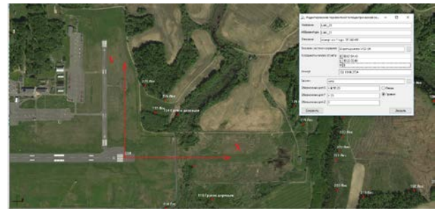
Figure 5 The local topocentric coordinate system
