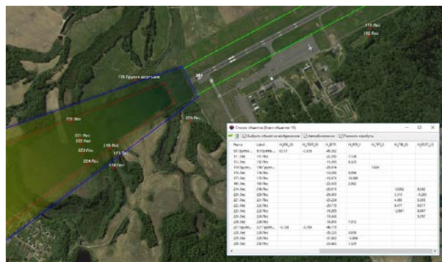
Figure 4. The take-off climb surface 3D dense model and a vector attribute structure
