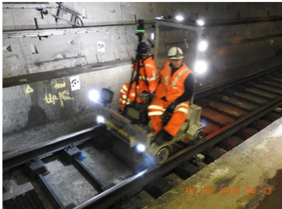
Figure 1. Test setup: camera mounted on the aluminium frame at the back of the vehicle together with the lighting system and laser scanner positioned between the two operators
