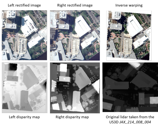
Figure 5. Left and middle: Outputs of our ground truth pipeline produced from the US3D JAX_214_008_004. Right: inverse warping and input lidar raster. This pair obtains the worse mean disparity error on buildings class according to SIFT (0.71 pix). Time discrepancy is visible on roof tops and a little on ground. Top left building in the left disparity map also shows an example of façade reconstruction from the nadir lidar.
