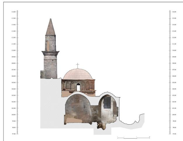
Figure 4. Drawing of a vertical transverse section.
