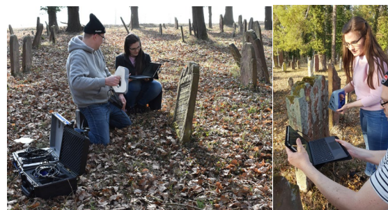
Figure 7. Handheld scanning handheld structured light scanner with Artec EVA (left) and Artec Spider (right),
