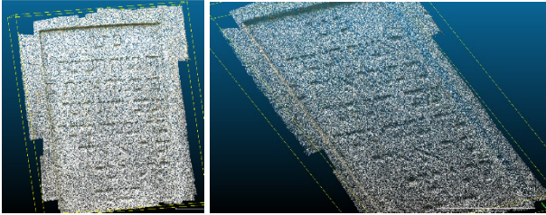
Figure 8. Examples of gravestones captured with BLK 360 laser scanner.
