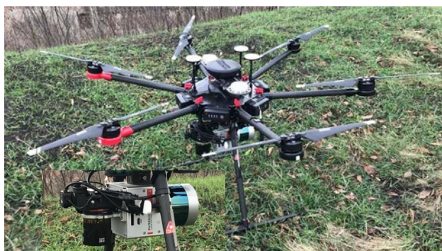
Figure 10. Integrated aerial mapping system
