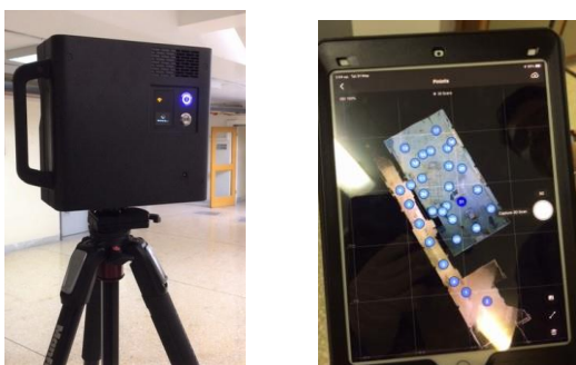
Figure 3. Matterport Pro2 3D and the display of data in the app during the acquisition
