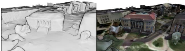
(b) Reconstructed mesh using our reconstruction method Figure 7. Left: shaded mesh model. Right: textured mesh model.
