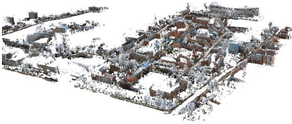
Figure 5. Dense reconstruction using our MetricSFM for two thirds of the campus region, totalling 7 billion color points.
