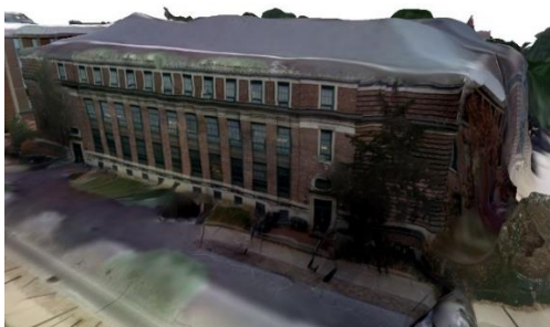
Figure 3. An example of the textured meshes reconstructed from our propose pipeline using both satellite and street-view data.
