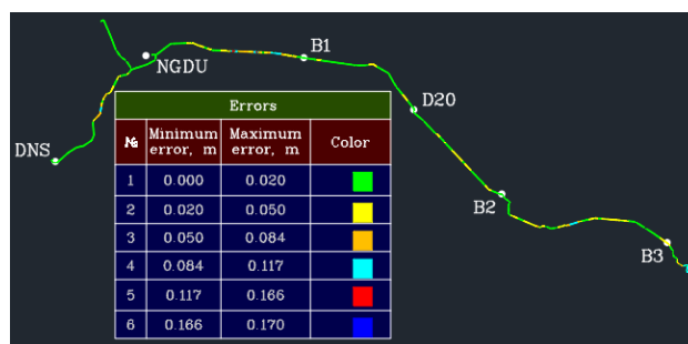
Figure 8. Error distribution for MLS data adjustment using check points every 1 km and control points every 8 km
